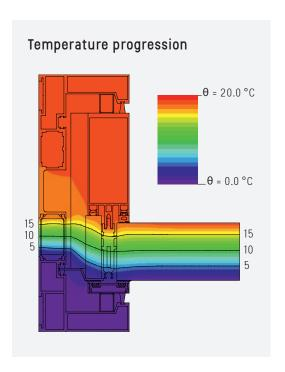
**Best heat insulation:** You save energy with the new HIRT SF XL. Best thermal insulation and the effective air exchange without room cooling are major features. Highly insulated aluminum profiles with 54 mm insulation stays and a  $U_f$  value of 1,418 W/m²K. Function glasses up to max 70 mm can be installed. HIRT SF XL values (examples): Size 6 x 3 m, 3-times glass U 0,5 W/m²K: The thermal transfer value of the entire descender front is  $U_W$  0,75 W/m²K.
