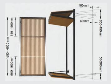
The shutters can be configured in a variety of ways including two leafs sliding upwards, biparting vertically and biparting with one leaf opening down and two folding upwards.
